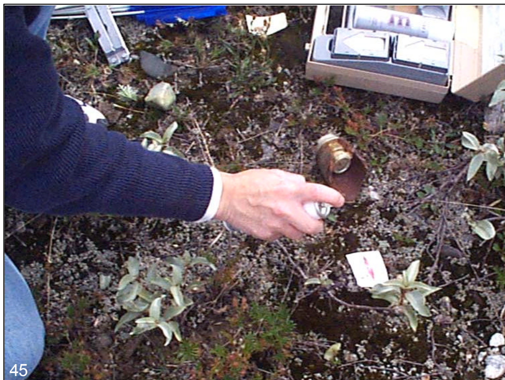
45 Sampling a piece of partially detonated ordnance for residual explosive. Color shows explosives present.
