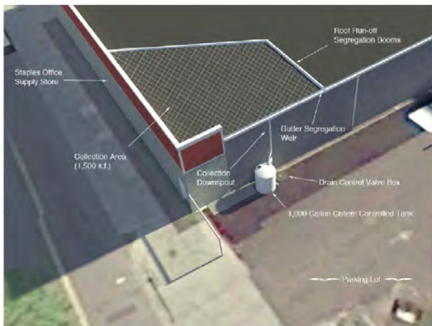
Photo 2-22. Cistern for Rainwater Harvesting
